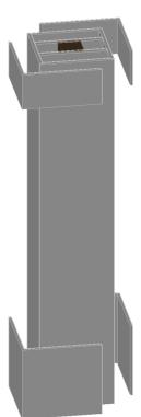
base around the column. Secure the cap and base with a finish nailer or trim screws.
