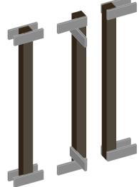
**Step 3:** Slide the L-shape half around the structural support & position as desired. Secure the half of the column to the post & blocking w/ galvanized or stainless-steel screws or finish nails (screws are recommended because the column shaft can be repositioned if necessary).
