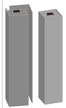
Step 4: Apply a continuous 1/4" bead of urethane adhesive caulk (included) along both mitered edges of the column half. Use a pneumatic finish nailer or stapler to fasten the two halves every 6"-8" along both sides of the column wrap. NOTE: Clean off any caulk squeeze-out with a clean, damp rag.
